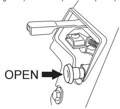
Figure 25. Choke Lever (Open Position)
